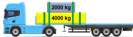
Partially against headboard: 1.5x weight of load (9000 kg) restraint
