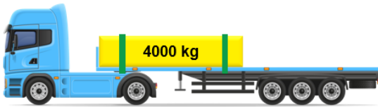
Against headboard: weight of the load (4000 kg) restraint
