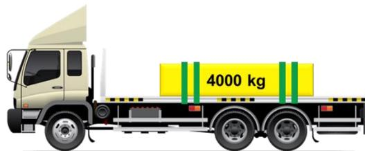
**Not against headboard:** twice the weight of the load (8000 kg) restraint
