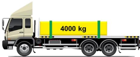
**Against headboard:** weight of the load (4000 kg) restraint
