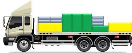
Load for correct axle weight distribution
