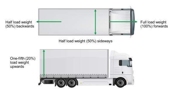
It requires much more force to stop a load that has started moving than it does to prevent the movement in the first place. It is essential that the vehicle is loaded and restrained so no part of the load can freely move in any direction.
