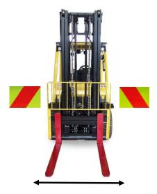
Max total width **2.55m** or **1.275m** from the longitudinal centre line If the load extends more than **200mm** on either side of the forklift, hazard warning signs must be used.
