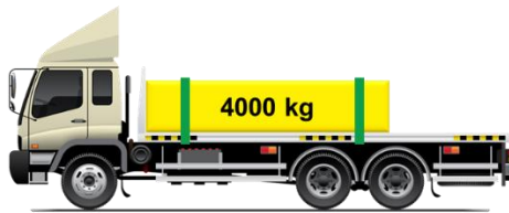
Against headboard: weight of the load (4000 kg) restraint
