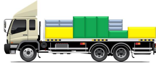
Load for correct axle weight distribution
