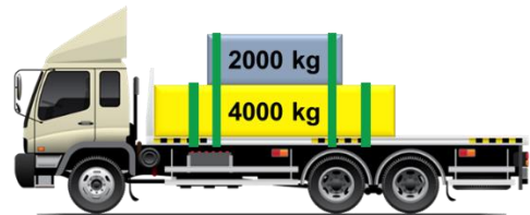
Partially against headboard: 1.5x weight of load (9000 kg) restraint
