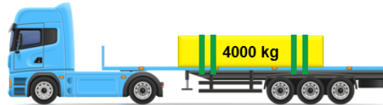
Not against headboard: twice the weight of the load (8000 kg) restraint
